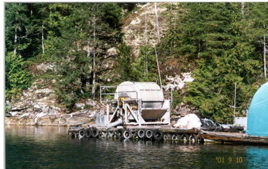
On-site net cleaning drum system
