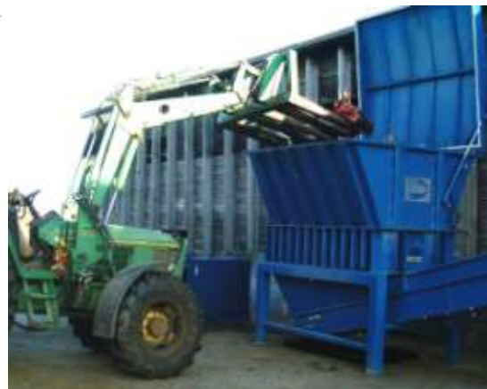
Canal Farms Grinder Being Loaded
