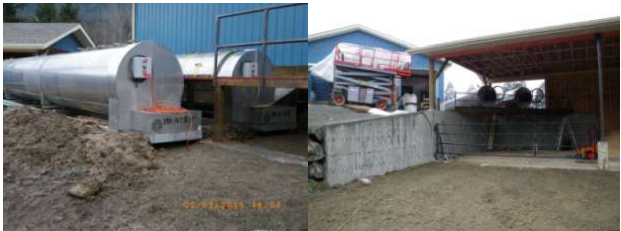
Tarzwell Farms Biovators in Place Ready to dump Non-SRM Composted Waste into Covered Holding Area
