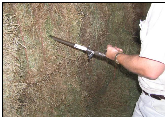
Figure 2. Collecting a core from a square bale
